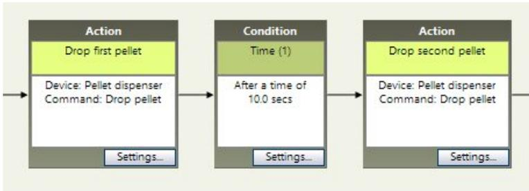
If the pellet dispenser is almost empty, it may take up to 30 seconds to deliver a pellet. make sure that the time specified in the Time condition exceeds the time that it takes the action to be carried out.
