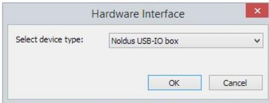
**TIP** To know what type of USB-IO box you have, check the label at the bottom side of the IO-box: PTIO-002x (for the Noldus USB-IO Box) or PTIO-003x (for Noldus Mini USB-IO Box).
